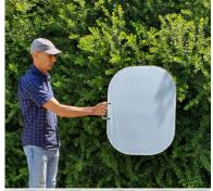
The picture on the left is an example of how not to use the ST, it has vegetation in the background. Vegetation temperature is usually very close to ambient air temperature.
