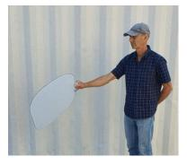
The picture on the left shows how  $\underline{not}$  to hold the ST – it is not perpendicular to the line of sight of MetCam.
