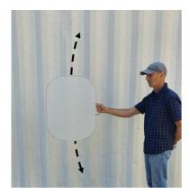
Swing the ST up and down as described in the photo on the left. The stroke of swing should be large and each swing should take 1-2 seconds. Don't swing it too hard – it will break the ST.
