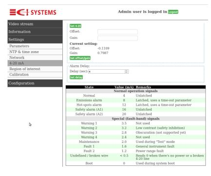
A table with the different 4-20 levels, used by MetCam, is displayed here for convenience.
