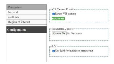
Inhibition in MetCam means that 4-20 mA alarm signals, related to Safety, are disabled.
