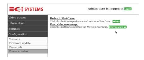
Do not skip the warmup in cases where the system is powered up – allow it to complete its 30 min.
