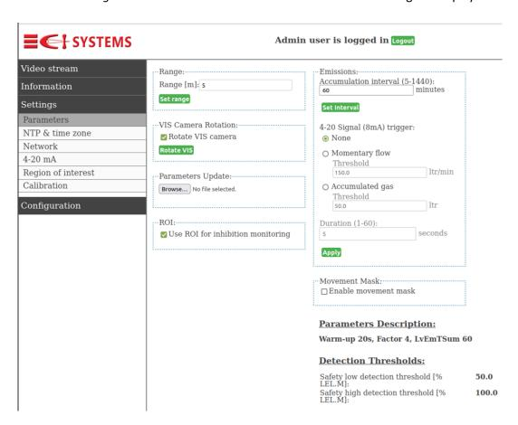
Insert the range, in meters, to the main monitored object/area. This data will be used to calculate gas cloud size.
