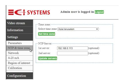
This interface allows a user to define the address of a local network NTP server. This setting survives power cycles and so will keep MetCam time correct even in the event of one.
