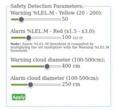
For a Warning or Alarm signal to be produced (16 or 20 mA), a gas cloud needs to be both denser and larger than the set values
