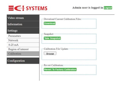
**Download Calibration Files** – pressing this button will download all calibration files to the connected PC. This operation is needed when a change to any existing file is needed due to specific installation conditions.
