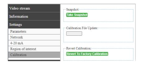
Pressing the *Take Snapshot* button will capture and download to the connected PC, a zip file containing these two images. These images can then be used to improve image registration, especially in cases where the monitored area distance is less than 5 meters or in cases where the monitored area includes objects at a large diversity of ranges.
