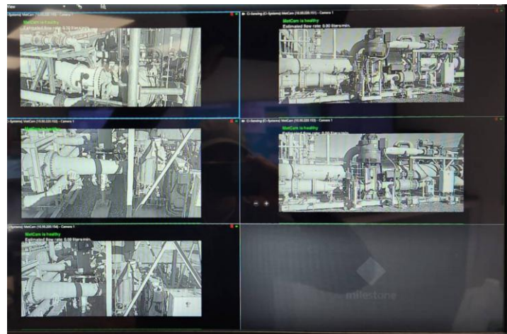
MetCam live output videos displayed on an ONVIF client application in the site control room
